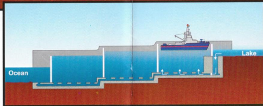
*A complex system of culverts and valves controls the level of water required to elevate and lower the ships inside the locks.*
